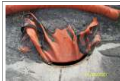
Gap allowing sediment to enter
